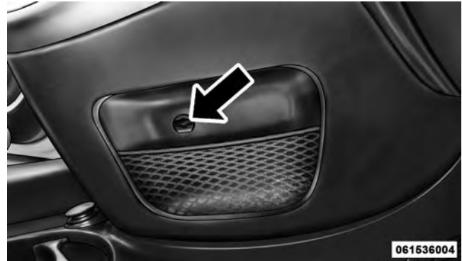
Shift Lever Override Access Hole
