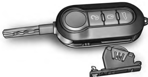
Battery Case Removed
