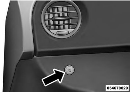
ESC Off Switch (Manual Transmission)
