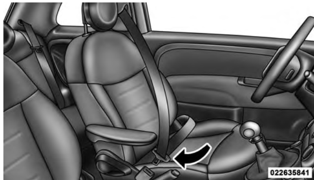
Inserting Latch Plate Into Buckle
