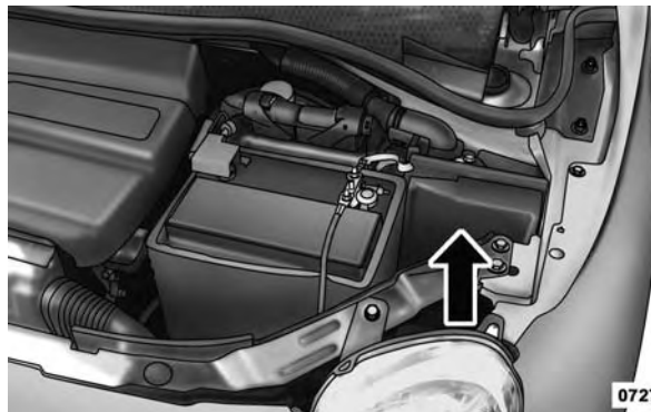
Front Distribution Unit
