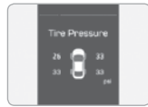
Low Tire Pressure Position Indicator and Tire Pressure Indicator (Shown on the LCD display)
