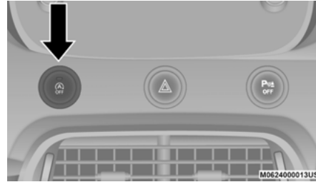
Stop/Start OFF Switch
