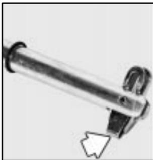
4. Push the clip so it locks in place. Pin is shown off of the vehicle for clarity.
