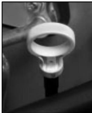
The engine oil dipstick has a loop handle and is located on the passenger’s side of the vehicle. See “Engine Compartment Overview” in the Index for more information on location.
