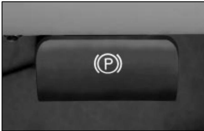
To release the parking brake, hold the regular brake pedal down. Pull the bottom edge of the lever, located above the parking brake pedal to release the parking brake.
