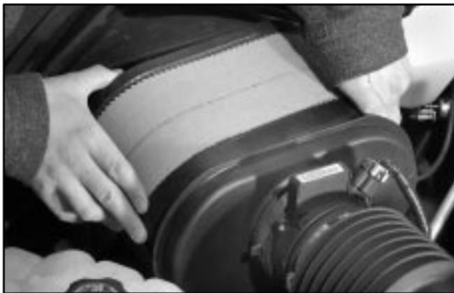
2. Pull the air cleaner/filter up and out from the housing. Care should be taken to dislodge as little dirt as possible.
