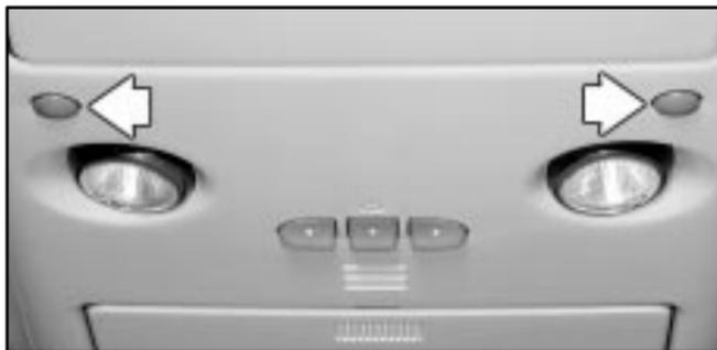
Your vehicle has front reading lamps located in the overhead console. Press the round button located next to the lamp to turn the lamp on. The lamps can be adjusted to point in the direction you want them to go.
