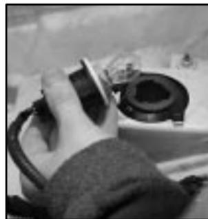
2. Turn the bulb socket counterclockwise and remove it from the lamp housing.
