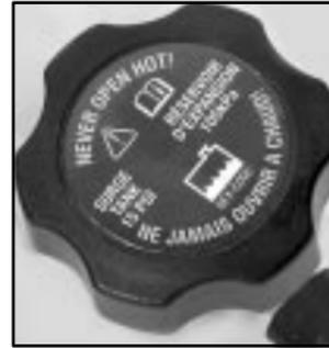
5. Then replace the pressure cap. Be sure the pressure cap is hand-tight and fully seated.
