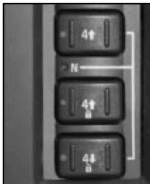
The transfer case buttons are located to the right of the steering wheel on the instrument panel. Use these buttons to shift into and out of the different all-wheel drive modes.
