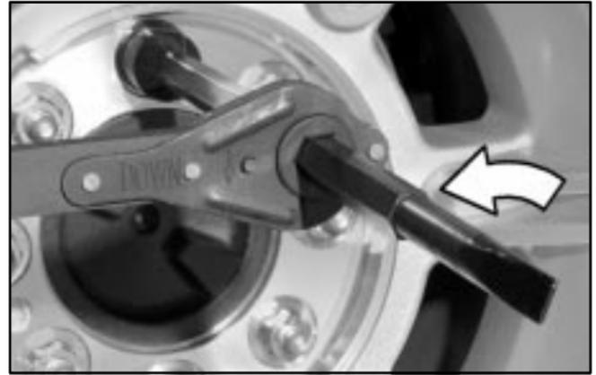
2. Slide the ratchet onto the wheel wrench with the DOWN mark facing you.
