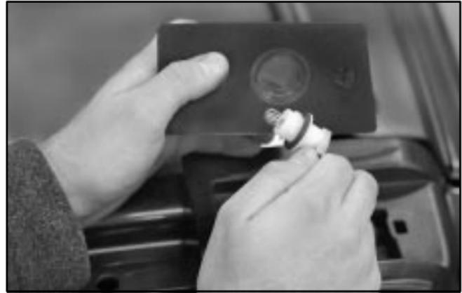
2. Turn the socket counterclockwise to remove it and remove the old bulb.
