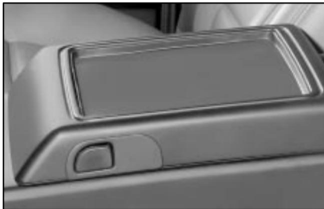
To open it, press the button on the side and swing the console lid open. The console includes CD holder slots and a tissue holder which is located on the inside of the console lid.
