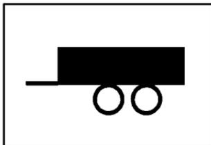
When the button is pressed, this light on the instrument panel will illuminate to indicate that tow/haul has been selected.
