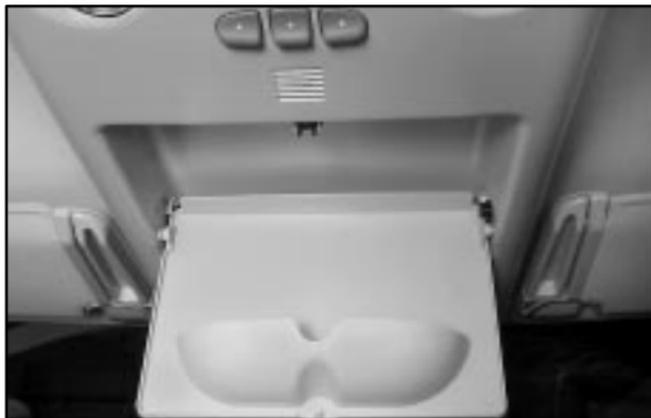
To open a door on the long console, push on the rear edge of the door and let it swing open. Push the door up until it latches to close the door.
