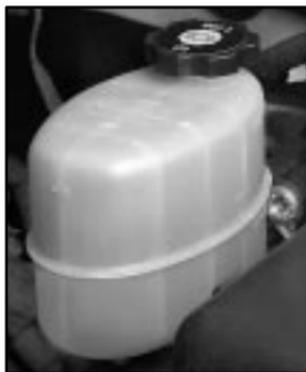
Your brake master cylinder reservoir is filled with DOT-3 brake fluid. See “Engine Compartment Overview” in the Index for the location of the reservoir.
