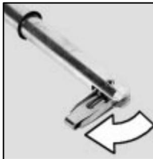
3. Turn the clip so that it is perpendicular to the pin. Pin is shown off of the vehicle for clarity.
