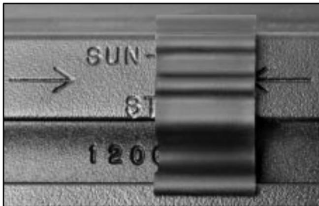
If your vehicle has a sunroof, it will have crossrail stop tabs placed in the siderails. These tabs prevent you from moving the crossrails past the opening of the sunroof and loading cargo too far forward. Cargo loaded too far forward could fall onto the sunroof and into the passenger compartment. Loading cargo too far forward could also cause the OnStar and navigation system (if equipped) to function improperly or not at all.
