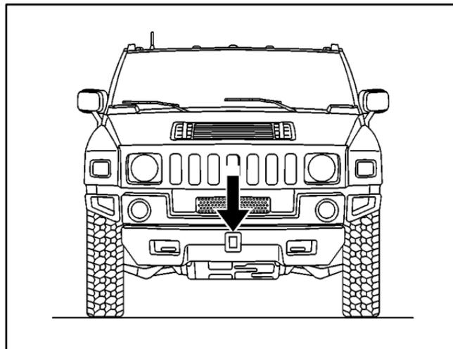
Your vehicle is equipped with a front receiver.
