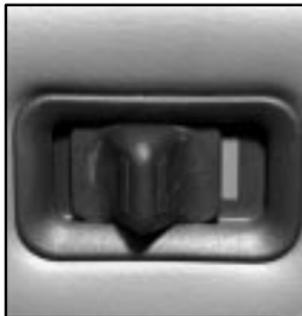
You can lock or unlock the door from the inside by sliding the manual lever forward or rearward. When the door is unlocked, you can see a red area on the lever.
