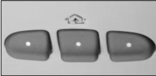
HomeLink, a combined universal transmitter and receiver, provides a convenient way to replace up to three hand-held transmitters used to activate devices such as gate operators, garage door openers, entry door locks, security systems and home lighting. Additional HomeLink information can be found on the internet at [www.homelink.com](http://www.homelink.com) or by calling 1-800-355-3515.
