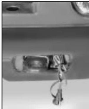
3. Plug it into a normal, grounded 110-volt AC outlet.
