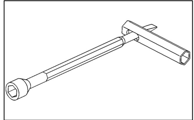
2. Place the flat end of the wheel wrench through the hole in the spanner wrench.
