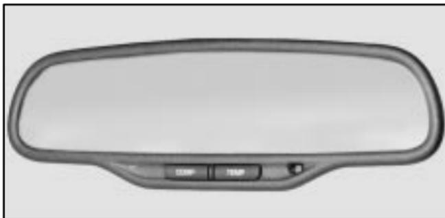
The mirror also includes a dual display in the upper right corner of the mirror face. The compass reading and the outside temperature will both appear in the display at the same time.
