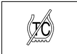
The TRAC OFF light will come on when a Traction Control System, Anti-Lock Brake System or engine-related problem has been detected and the vehicle needs service.
