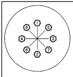
11. Tighten the nuts firmly in a crisscross sequence as shown by turning the ratchet clockwise, with the UP mark facing you.
