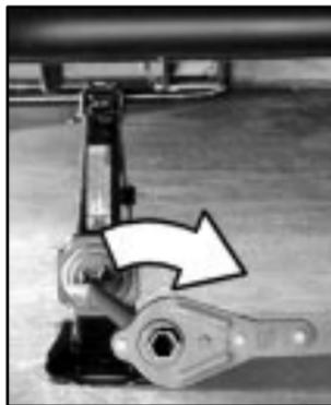
**Front Flat Tire:** Position the jack under the vehicle on the frame behind the flat tire where the frame sections overlap. See the graphic following for an approximate measurement of the jack location on the frame.
