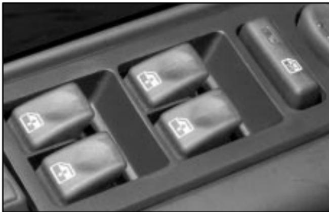
The driver's door has a switch for each of the passenger's windows as well.
