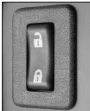
On the passenger side of the liftgate opening trim there is another power lock switch which can be used to lock or unlock all of the doors.
