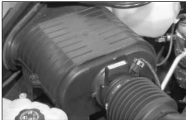
The engine air cleaner/filter assembly is located in the engine compartment on the passenger's side of the vehicle. See "Engine Compartment Overview" in the Index for more information on location.
