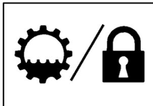
The transmission dipstick handle is located at the rear of the engine compartment. Your vehicle's dipstick may have a graphic as shown or may be labeled **TRANS/LOCK**.
