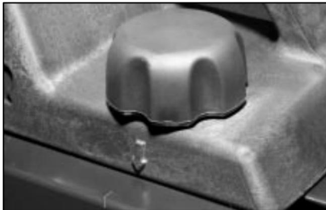
1. Loosen the lock knobs on the crossrail support by turning the knobs counterclockwise. Only loosen them enough to allow the crossrails to slide easily.
