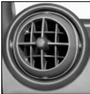
Your vehicle has air outlets that allow you to adjust the direction and amount of airflow inside the vehicle. Push the knob up, down, left or right to direct the airflow. Increase or decrease the amount of air flow by turning the knob, located in the center of the vents.
