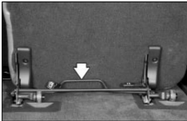
4. Squeeze the release handle while pulling the seat out.
