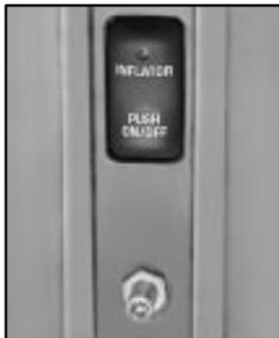
The air inflator is located in the rear compartment on the passenger's side of the vehicle.
