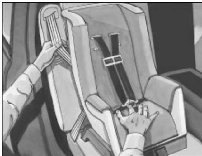
6. To tighten the belt, feed the shoulder belt back into the retractor while you push down on the child restraint. If you're using a forward-facing child restraint, you may find it helpful to use your knee to push down on the child restraint as you tighten the belt.
