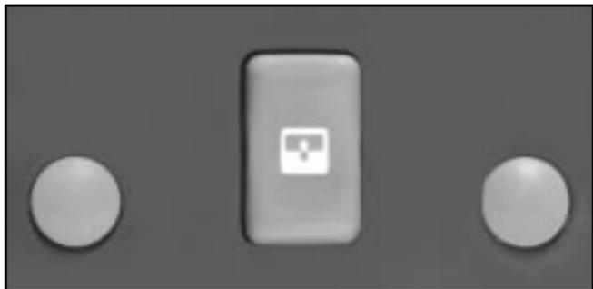
To open the sunroof and sunshade, press and hold the rear side of the button, located on the overhead console, until the sunroof reaches the desired position or until it stops at the built-in comfort position. The comfort position stops the sunroof from opening completely.
