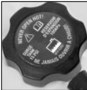
The coolant surge tank pressure cap must be fully installed on the coolant surge tank.
