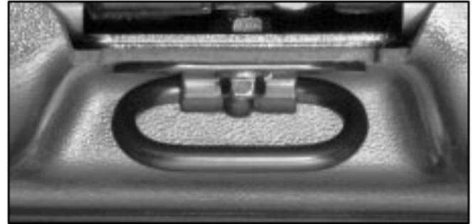
There are two cargo tie downs located on the inside of the liftgate in the rear of the vehicle to secure cargo inside the vehicle with the liftgate closed.
