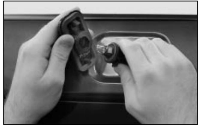
2. Turn the bulb socket counterclockwise and remove it from the lamp housing.
