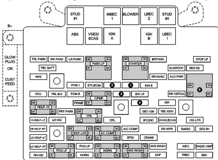
\* NOTE: The function and amperage of these fuses are different for gas and diesel fueled engines. See Owners Manual [1] for functions of studs #1 and #2.
