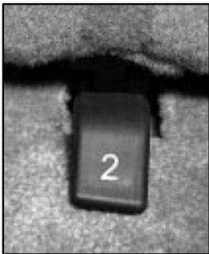
3. To unlatch the rear of the seat from the floor, pull up on the release lever labeled 2, located at the rear of the seat, and lift the rear of the seat up off of the floor.
