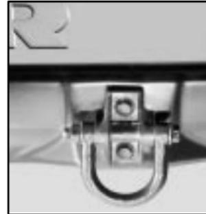
Your vehicle is equipped with recovery loops at the front and rear. You may need to use them if you’re stuck off-road and need to be pulled to some place where you can continue driving.
