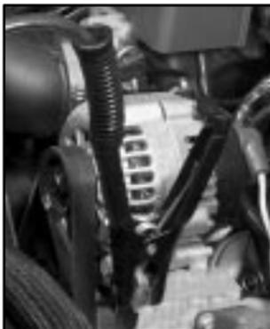
9. Connect the other end of the negative (-) cable to the remote negative (-) terminal, marked GND, on the vehicle with the dead battery.
