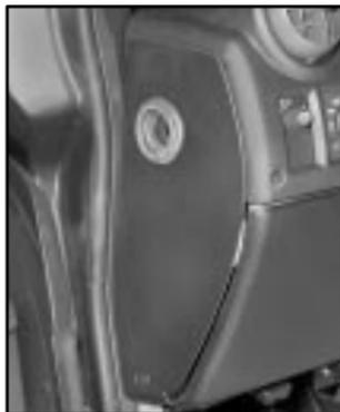
The fuse block access door is on the driver's side end of the instrument panel. Pull off the cover to access the fuse block.
