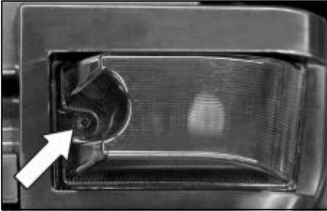
1. Remove the screw and lift off the lens.
