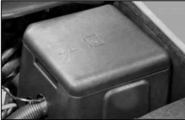
The underhood fuse/relay block is located near the battery in the engine compartment. See “Engine Compartment Overview” in the Index for more information on its location. Lift the cover for access to the fuse/relay block.
