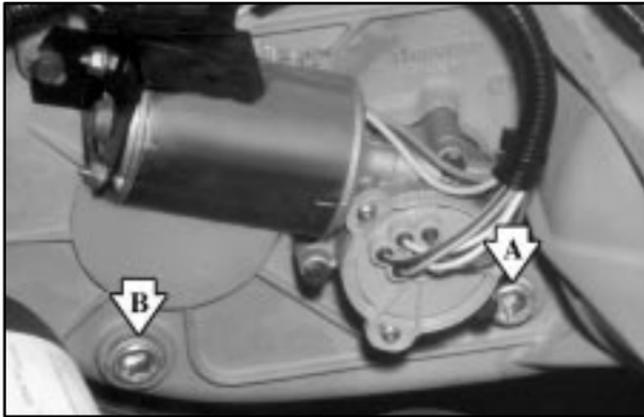
(A) Fill Plug (B) Drain Plug
