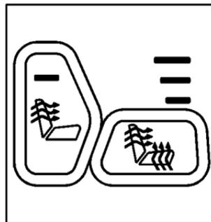
The buttons for the driver's side heated seat are located on the driver's side door panel. The buttons for the passenger's side heated seat are located on the passenger's side door panel.
