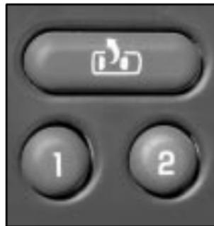
The controls for the memory function are located on the driver's door trim panel.
