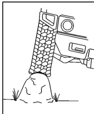
*Roll Your Tires Over Large Rocks.* Do not straddle large rocks; drive over them, letting the tire envelop the rock. The tread of the tire is thicker and tougher than the sidewall of the tire and is more resilient to impact than underbody components.
