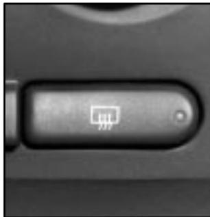
The lines you see on the rear window warm the glass. Press the button to start warming your window. A light will glow in the button while the defogger is working.
