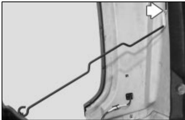
6. Pull the end of the prop rod from its holder and place it into the slot built into the hood.
