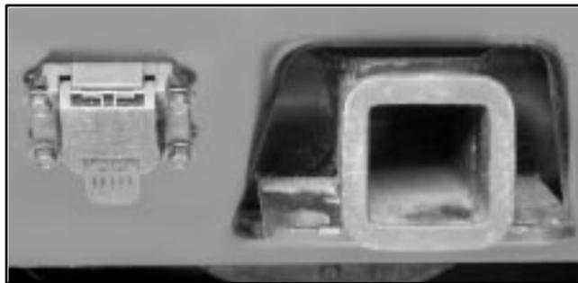
Your vehicle is equipped with the eight-wire trailer towing harness. This harness with a seven-pin universal heavy-duty trailer connector is attached to the rear bumper.
