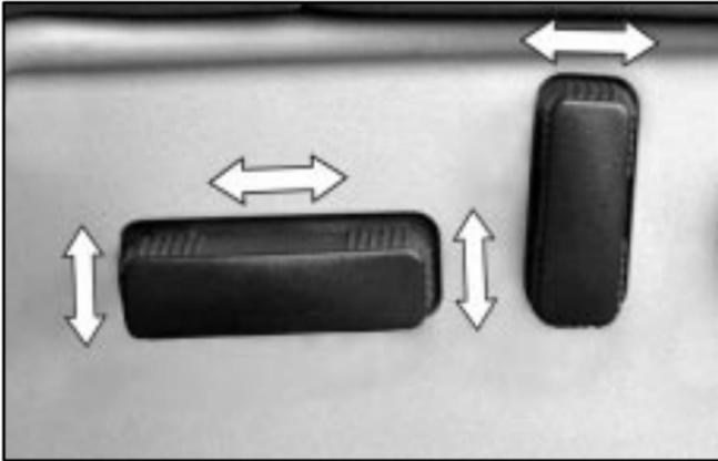
**Horizontal Control:** You can adjust your vehicle's front seats with the horizontal control located on the outboard edge of each front seat.
