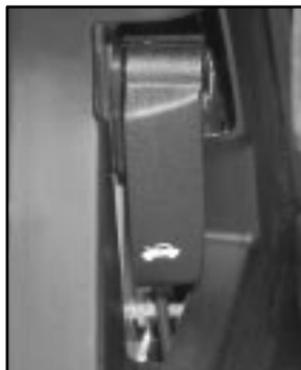
2. Pull the handle located on the lower part of the instrument panel.
