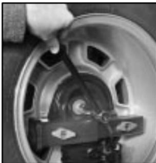
Then use the ratchet and spanner to tighten the nut firmly. Try to move the tire back and forth slightly to be sure it is secure.
