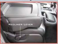
The front passenger seat can be folded flat to allow for extended cargo space.
