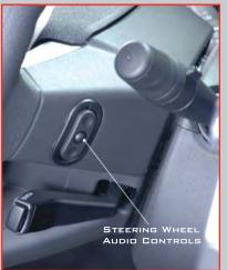
The steering wheel audio controls are located on the rear surface of the steering wheel.
