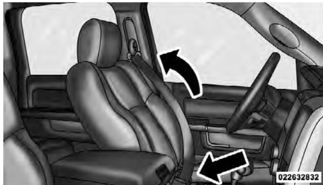
Removing Slack From Belt
