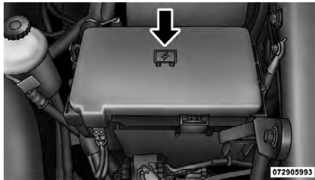
Totally Integrated Power Module
