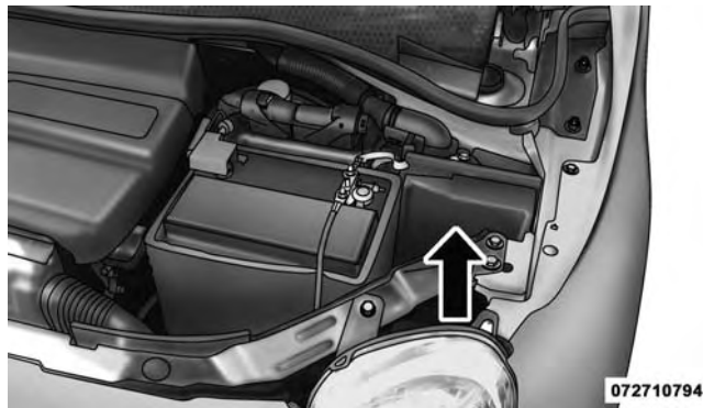
Front Distribution Unit
