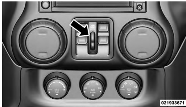
Window Lockout Switch
