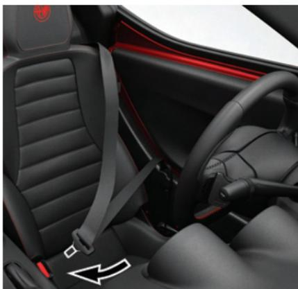
Inserting Latch Plate Into Buckle
