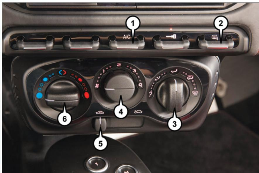
Heating/Ventilation And Air Conditioning Controls
